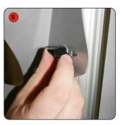
The linear post should have the bar and thumbscrews already attached. Unscrew the thumbscrews, and insert through the side of the literature holder, screwing back into the bar to secure
